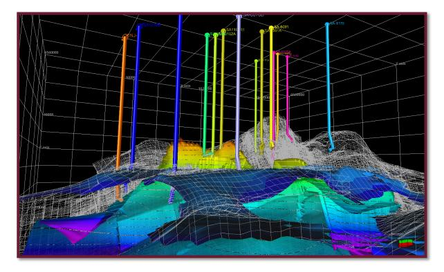
The horizontal well initiative has advantages over the vertical design in terms of greater reservoir contact, reduction of fracture flow and a greater volume of injection if necessary as long as the control devices in the background are available for correct administration of the injection... although it should be noted that this initiative is not imminent to take immediate actions for the indispensable redistribution of injection
