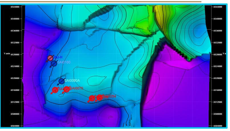
Due to the current situation in which some producing wells of the field are being invaded by injection water, a simulation was carried out in Petrel using the data of the static & dynamic models to define the preferential routes of the injected waste water to through the current injector wells by dividing them into two zones: southern periphery (red wells) and west zone...
