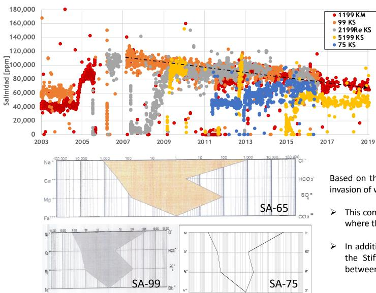
Based on the salinity of SA-65 and the behavior of neighboring wells, the invasion of water injection in the MC and LC is shown.
