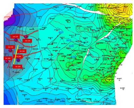
When injecting through a horizontal well, it is sought to have a more effective injection in an areal way, looking for a better sweep of oil that have been left behind by the channeling of water produced due to the high fracturing of the reservoir.
