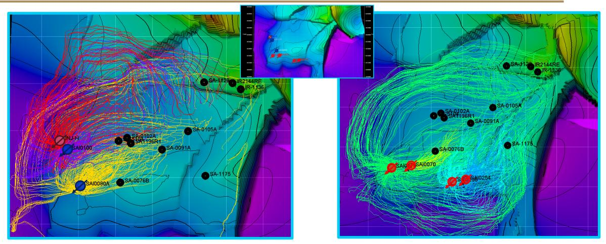
It is clearly seen that the preferential flow routes of the wells located in the southern peripheral zone tend to go towards the central and eastern part of the field, where precisely the highest percentage of producing wells is found, while the preferential flow routes of the Injection in the western zone are directed more towards the northern part, at the same time that they have much less influence in the area of producing wells\*\*.
