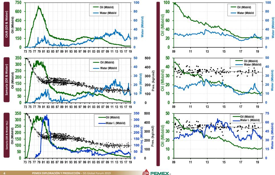
From the fields of the project, the importance of Samaria field can be observed, because 50% of the oil and water production of the project come from this field, in addition it is in this field where most of the wastewater is injected today. Therefore, the behavior in oil production is very similar with respect to the entire project.
