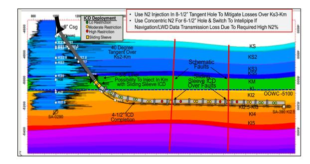
The flow controllers have capillary tubes with IDs that are defined according to the area and speed of the fluid required. Inflatable packers are used to insulate the areas of permeability variation identified.
