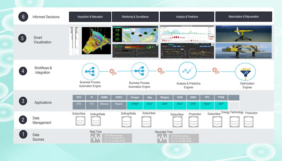
Data Flow Diagram shows how Live FDP system assimilate current softwares and integrate them within one ecosystem seemlessly
