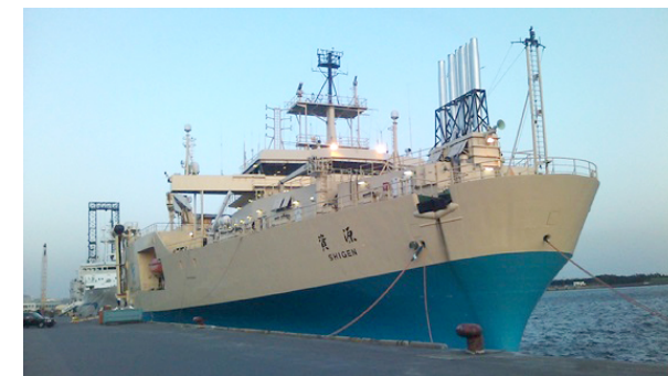
3D seismic vessel for domestic offshore survey
