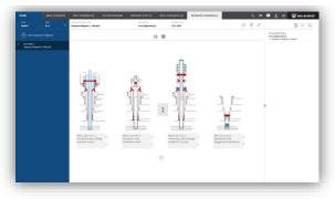
**Sequence Diagram** is a representation of selected well barrier illustrations you have prepared for the well. This can be output on A4, A3 or large size plotter paper and be made available in meeting rooms or places where all stakeholder have access and can see the planned progress of the well work.
