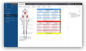
Well Barrier Schematic is the backbone of Wellbarrier Illustration Tool. The main purpose of the Well Barrier Schematic form is to show the well with all its well barrier elements in a clear and consistent manner.
