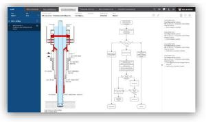
**Well Control Action** form has an easy to use flow diagram editor. It is used to show how well incidents can be handled.
