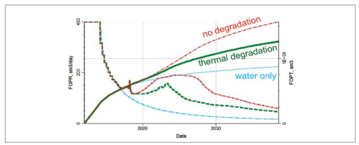
Effect of polymer thermal degradation on recovery.
