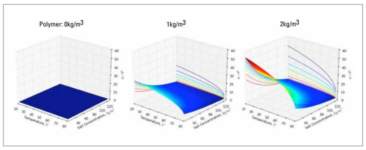
Polymer solution viscosity dependency on temperature and salinity.
