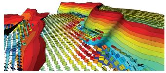
Modeled density and orientation of subseismic faults in reservoir from Poly3D forward stress modeling.
