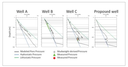
Wells A–C contain calibration data (measured pore pressure and mud-weight–derived pressure) and are from a pressure-calibrated 3D model. The plot on the right shows an extraction from the pore pressure model at a proposed well location.
