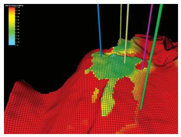
Overpressure distribution on a reservoir-scale model; high overpressure in rocks with low permeability (red), low overpressure in reservoir rocks (green).
