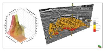
Litho classification and prediction from seismic inversion results. (Data courtesy of WesternGeco)
