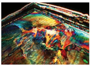
Generalized spectral decomposition result, RGB blended using the Mixer tool. (Data courtesy of Geoscience Australia)
