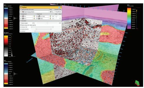
Mixer covisualization capabilities include flip/roll, RGB/CMYK blending, and masking. (Data courtesy of WesternGeco)
