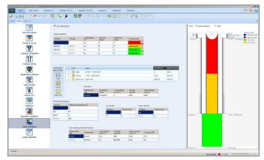
Model cleanup operations of a mud-filled well.
