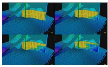
The ECLIPSE simulator supports modeling of numerous EOR options. Above is an example of a full-field polymer flood study.
