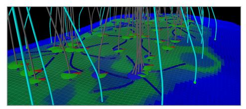
Full-field ECLIPSE simulation visualized with the Petrel E&P software platform.
