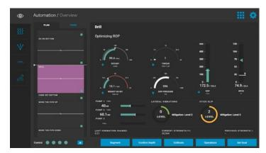
The DrillOps Automate dashboard provides the driller with an overview of activities and conditions.
