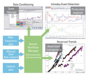
Avocet Workflow Manager data processing workflow. Data is acquired from multiple sources, then aggregated and conditioned to provide robust information for subsequent engineering analysis.
