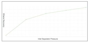
Effect of plant inlet separator on ethane recovery.
