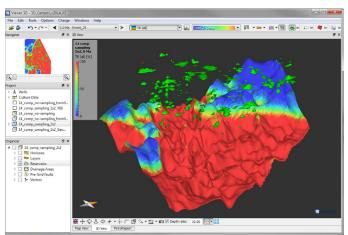
The PetroMod 3D core enables full 3D assessment of pressure and temperature in a sedimentary basin through geological time.
