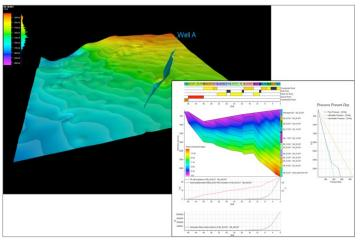
Geocellular models built in Petrel 2015 contain detailed facies and property distributions that can be incorporated into PetroMod software for dynamic forward modeling.
